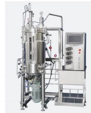
BLBIO-50SC 50L Bottom magnetic mixing fermentation system
