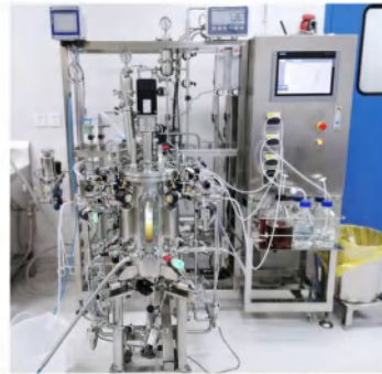
BLBIO-30SJA-FMT 30L Metabolic flow automatic bioreactor system
