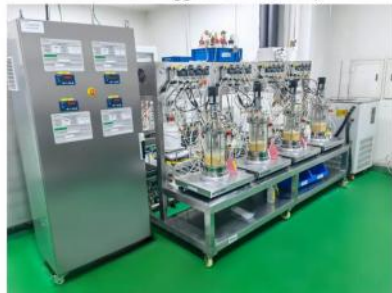
BLBIO-XGJ-4-plus Quadruple mechanical mixing glass fermenter (5L)
