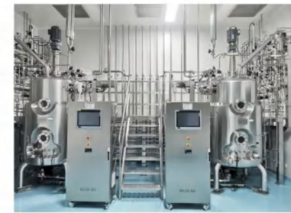
1000L Secondary Mammalian Cell Bioreactor
