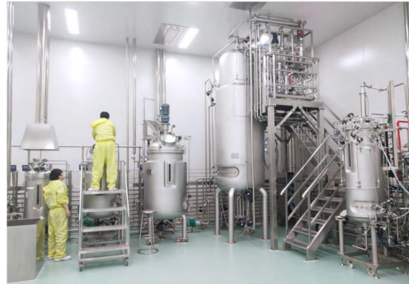
BLBIO-300S/JBA - 3000S/JBA 300L - 3000L Bottom mechanical mixing stainless steel fermentation system
