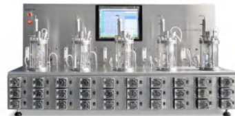
BLBIO-1GC-5-mini 1L quintuple magnetic multi-channel parallel bioreactor
