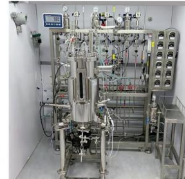
30L Bottom magnetic mixing bioreactor
