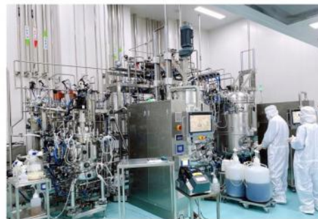
50L-800L Top magnetic mixing bioreactor
