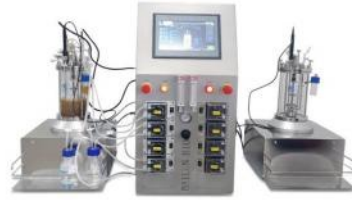
BLBIO-XGC-2-A Double magnetic mixing glass fermenter (desktop)
