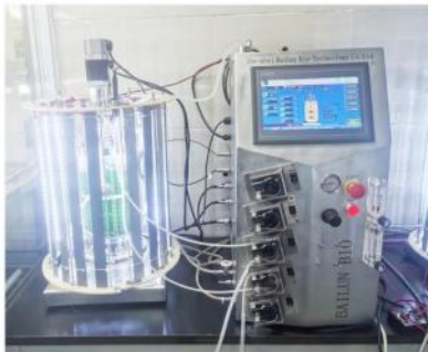
BLBIO-5GCL 5L Magnetic mixing photobioreactor (off-site sterilization)
