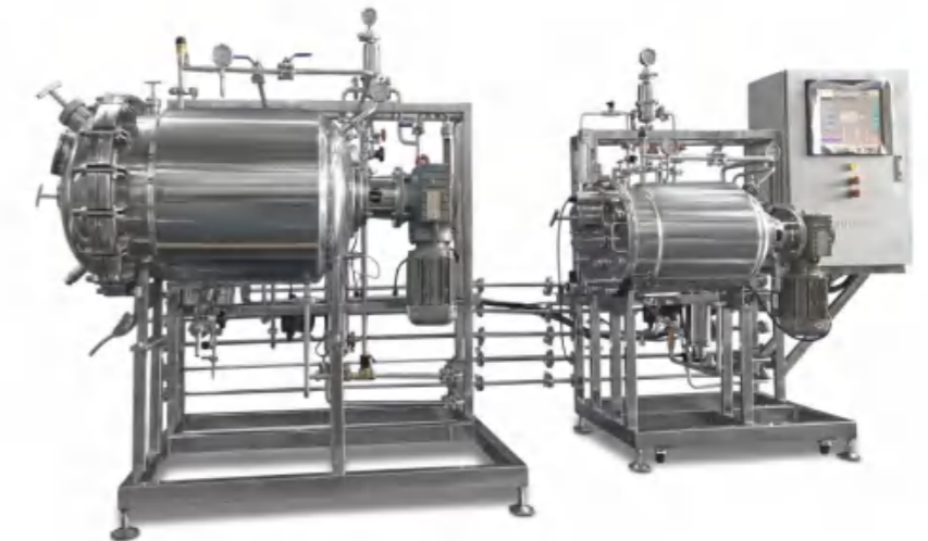
BLBIO-50SS-150SS 50L-150L Solid Secondary Fermentation System
