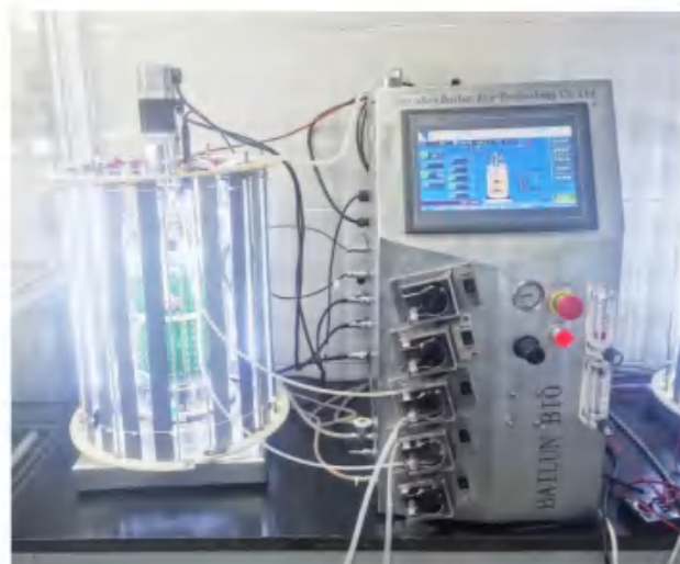
BLBIO-5GCL 5L Magnetic mixing photobioreactor (off-site sterilization)
