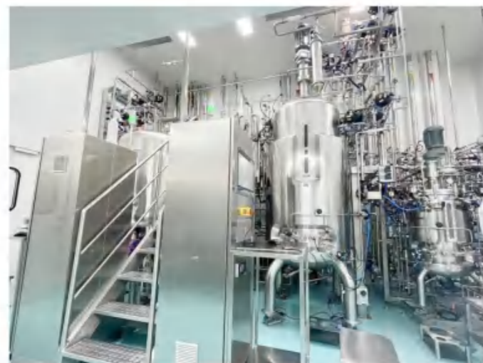
70L-1500L Top magnetic mixing bioreactor
