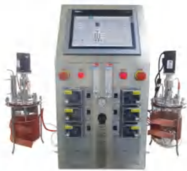
3L double cell bioreactor
