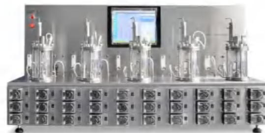
BLBIO-1GC-5-mini 1L quintuple magnetic multi-channel parallel bioreactor
