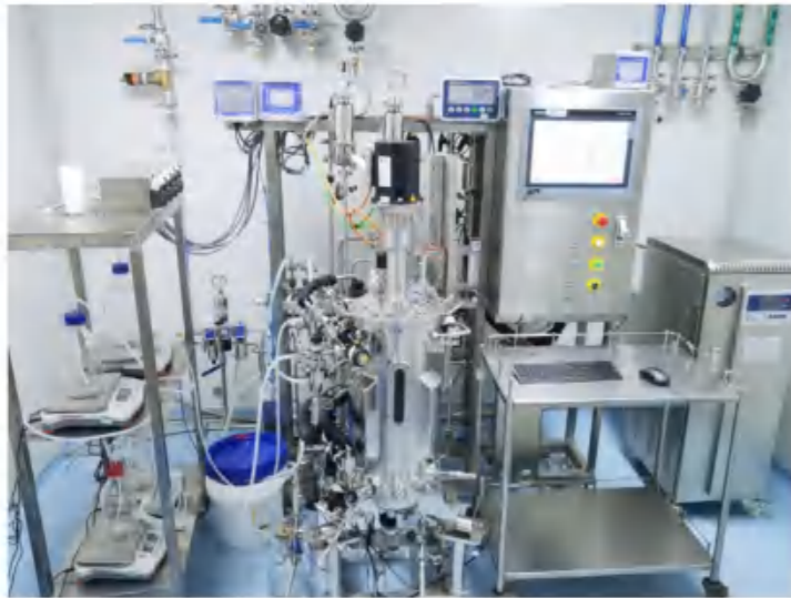
BLBIO-20SJA-FMT 20L Metabolic flow automatic bioreactor system
