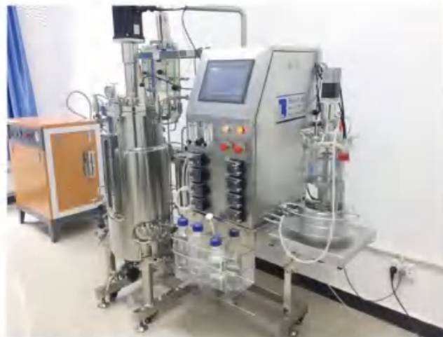
BLBIO-5GJ-50SJ 5L-50L Secondary Fermentation System
