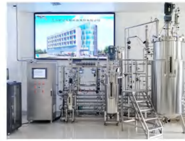
BLBIO-10SJD-100SJD-500SJD 10L-100L-500L Three stage fermentation system
