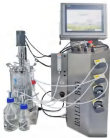
BLBIO-5GJ-plus Off-site sterilization shaft driving glass fermenter (mechanical stirring fermenter)
