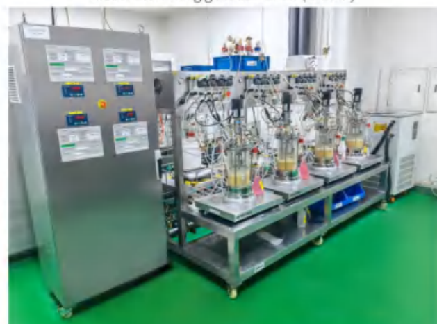
BLBIO-XGJ-4-plus Quadruple mechanical mixing glass fermenter (5L)
