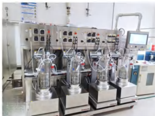
BLBIO-XGC-4-plus Quadruple magnetic mixing glass fermenter (5L)
