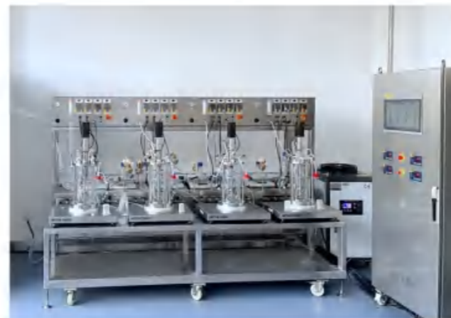
BLBIO-5GJ-4FMT 5L Quaduple metabolic flow automatic bioreactor system
