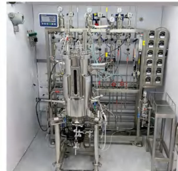
30L Bottom magnetic mixing bioreactor
