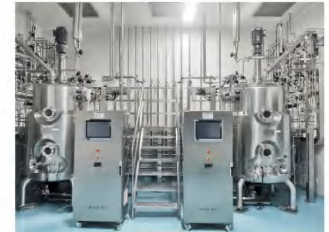
1000L Secondary Mammalian Cell Bioreactor
