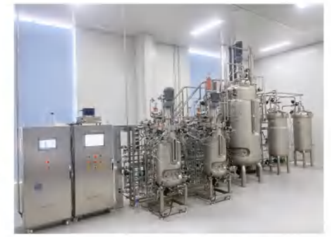
BLBIO-100SJA-100SJA-1000SJA 100L-100L-1000L Double secondary fermentation system
