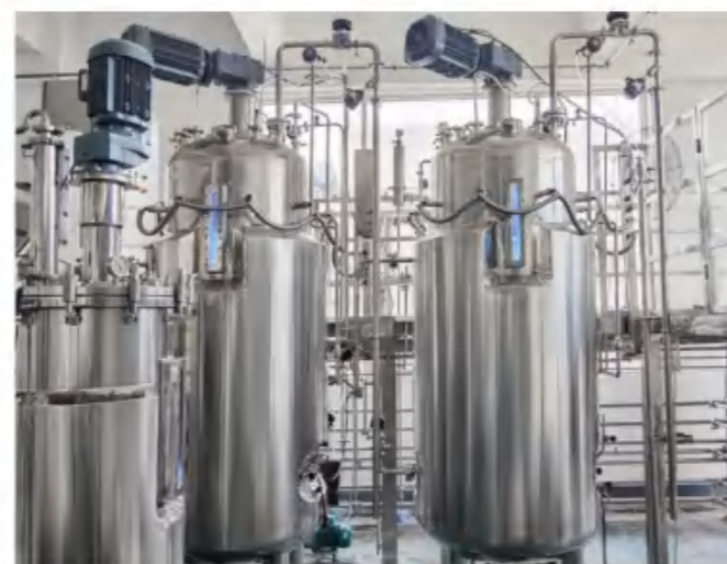
BLBIO-1000SJL-1000SJL 1000L Double stainless steel photobioreactor
