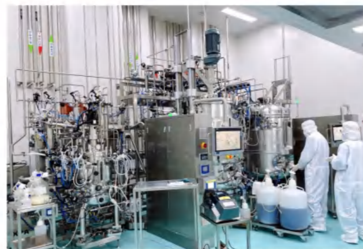
50L-800L Top magnetic mixing bioreactor
