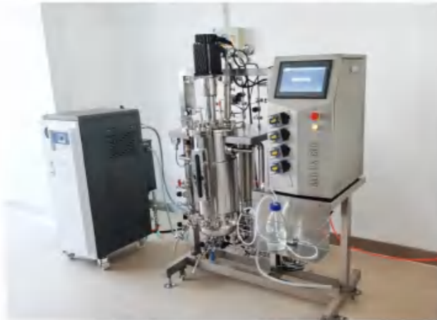
BLBIO-30SJA 30L Top mechanical mixing stainless steel fermentation system
