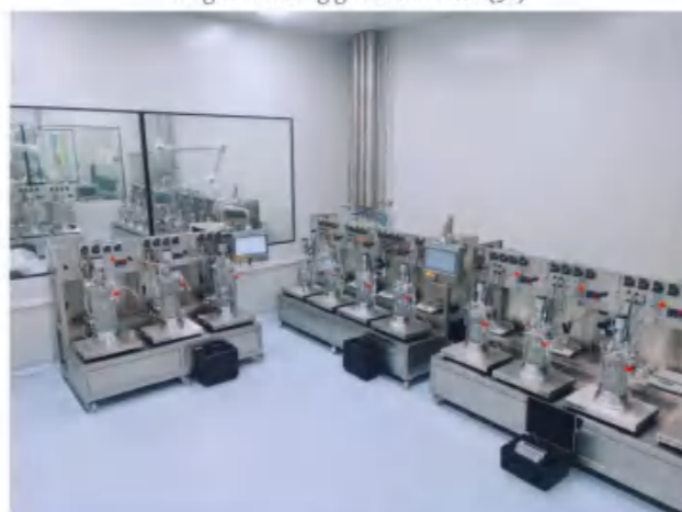
BLBIO-XGJ-11-plus Elevenfold mechanical mixing glass fermenter (5L)
