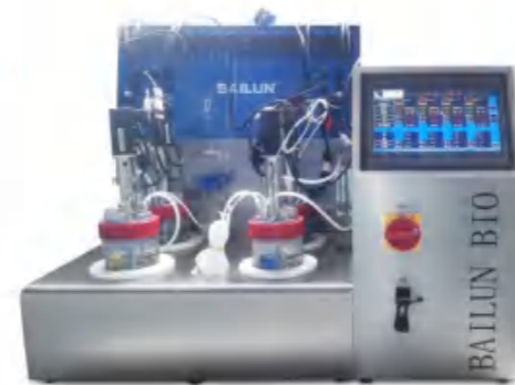
BLBIO-1GJ-4-mini 1L quadruple multi-channel micro-bioreactor
