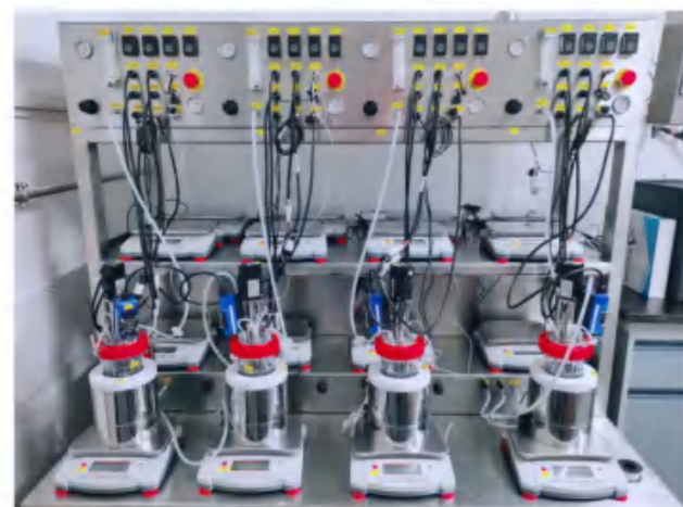
BLBIO-XGC-4-plus Quadruple mechanical mixing glass fermenter (500ML)
