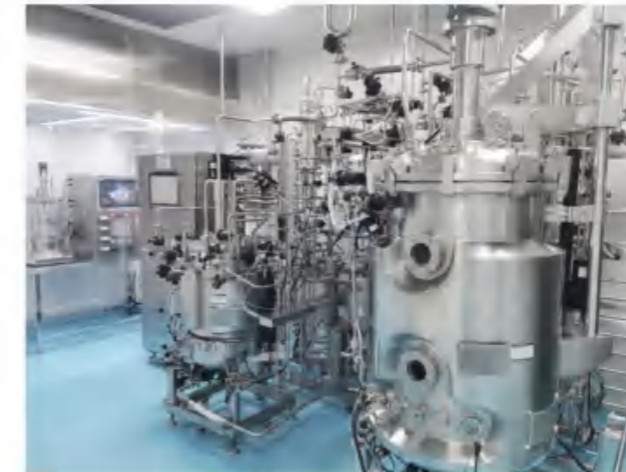
50L-250L Secondary Mammalian Cell Bioreactor
